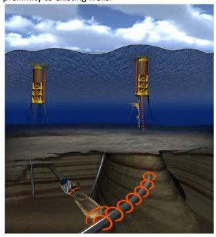
This method uses ClampOn non-invasive ultrasonic sensor technology in the form of a spectrum analyzer. The spectrum analyzer digitizes the ultrasound allowing frequency analysis in real-time. The procedure is patent pending.
